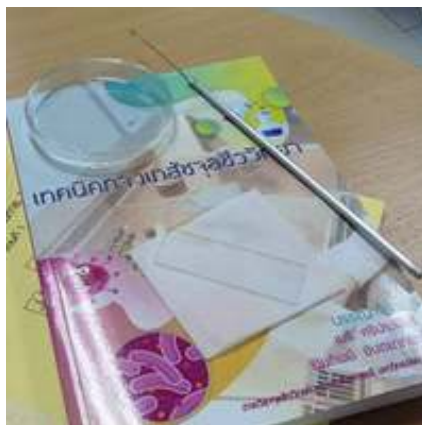
Figure 3. Manual of General Microbiology Laboratory along with glass slide, plastic petri dish and inoculation loop that were shipped to all second year students.
